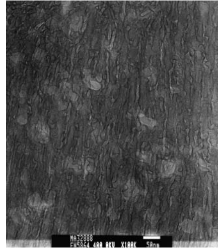
Figure 4: X100,000 TEM micrograph documents the microstructure of the composite finish. Note the differences in the microstructure as compared to the Type I and Type II finish microstructures. The composite microstructure appears as a hybrid of the two finishes.
